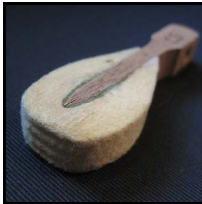
Hammer with significant wear.
