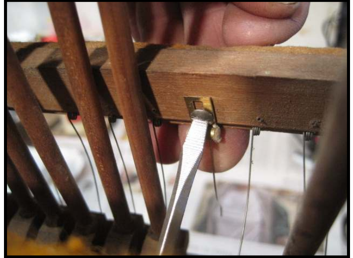
A hammer butt repair spring being installed.
