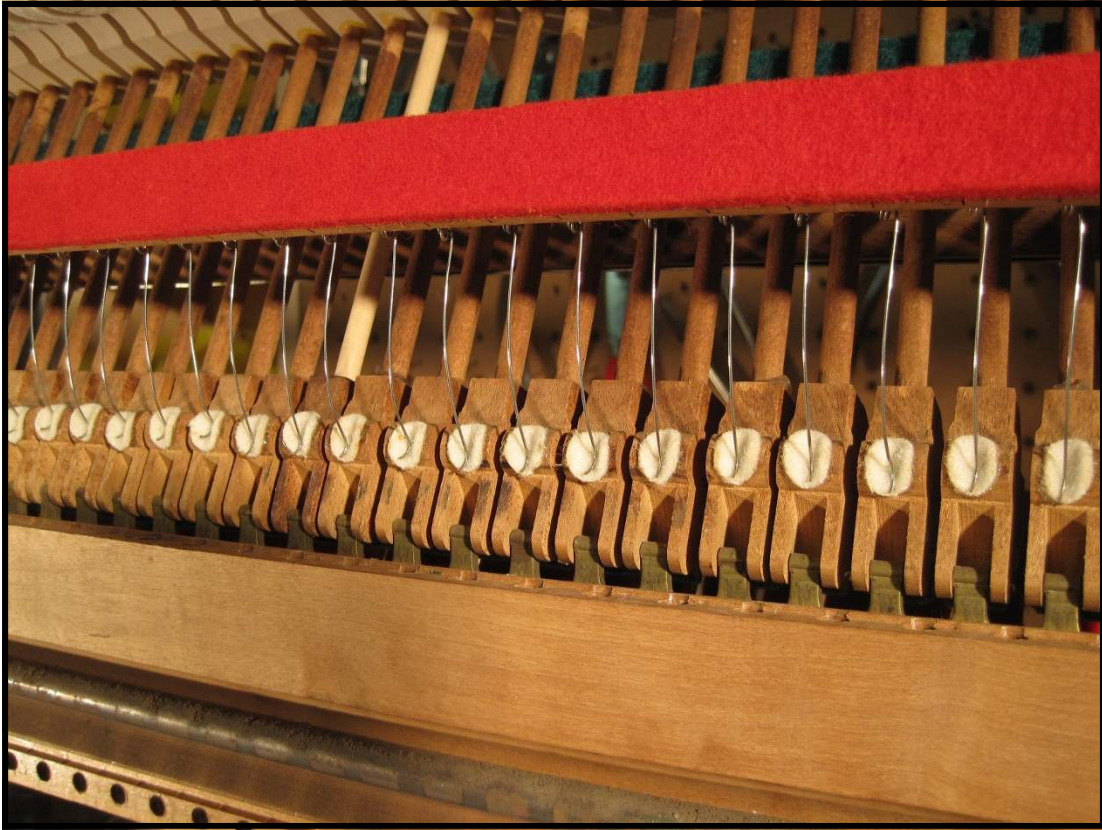
A net set of hammer rail springs helps complete an upright action restoration job.
