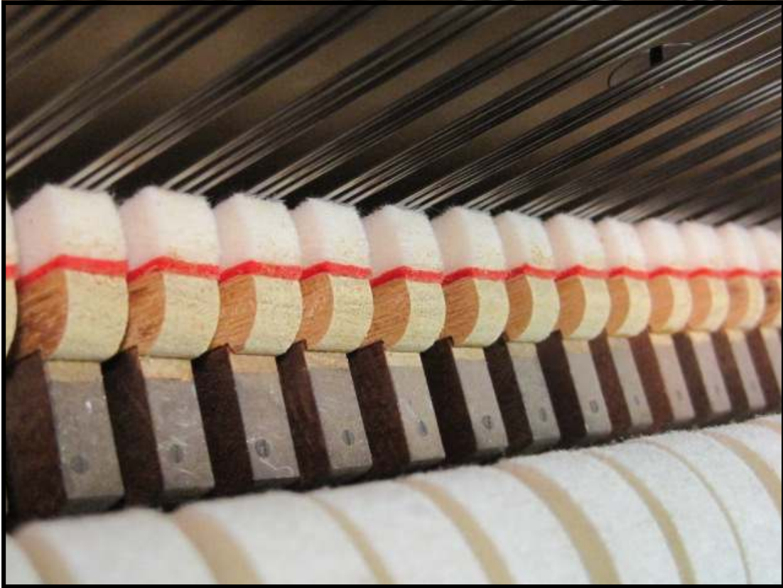
A new set of treble dampers installed and ready quiet things down when needed.
