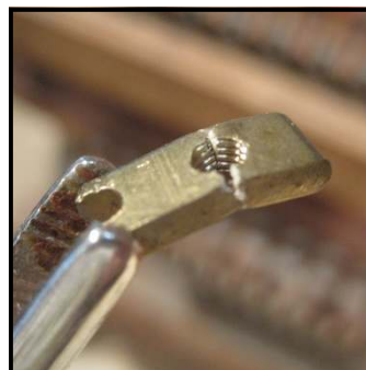
Broken butt plate
