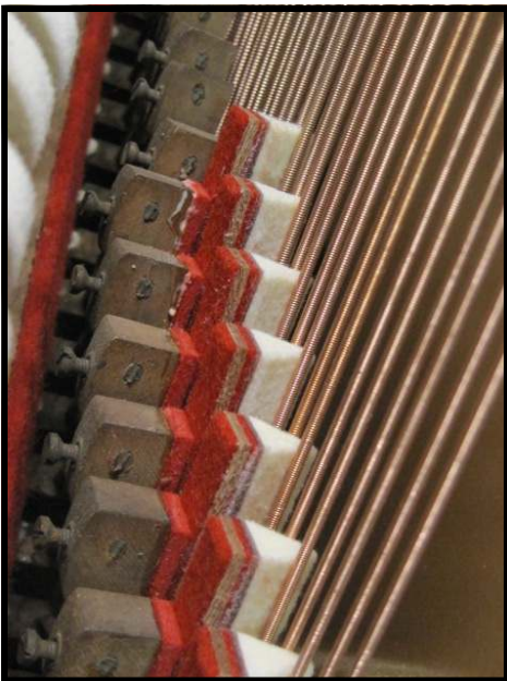
New bass dampers being installed.
