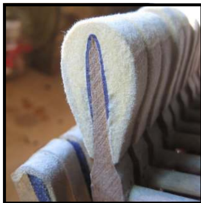
Worn hammer after filing
