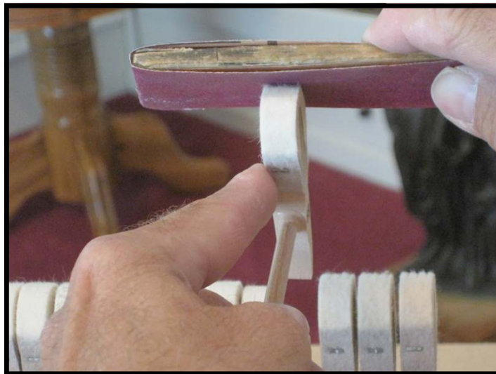
Hammers being filed to remove cut marks.
