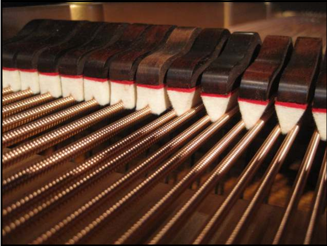
A new set of dampers installed and ready quiet things down when needed.
