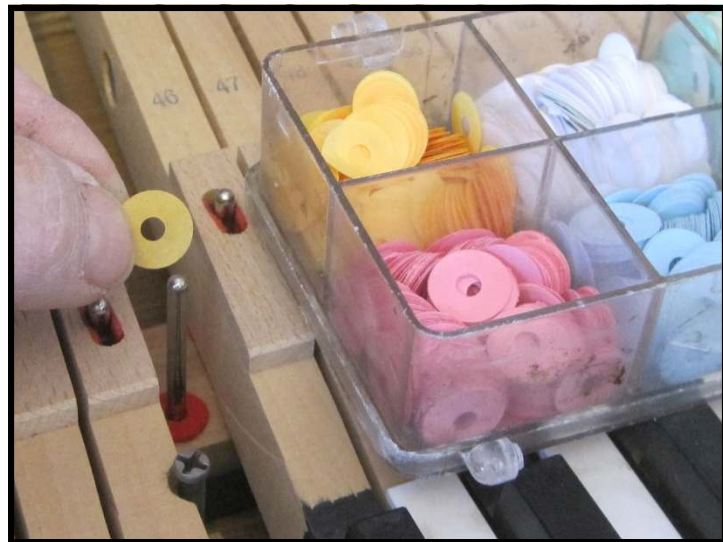
.002" paper punching being installed
