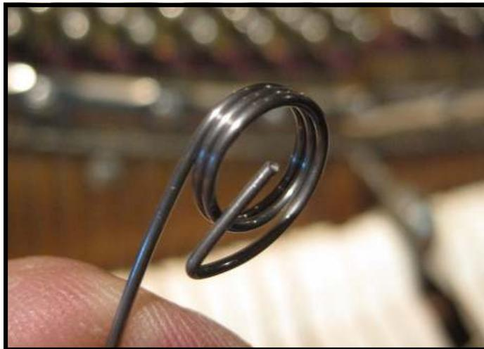
To splice a string, a new coil is first produced as shown in the above photo. A tuner's knot is then tied, splicing the new wire together with the old. This knot, when done correctly, will be a permanent fix.
