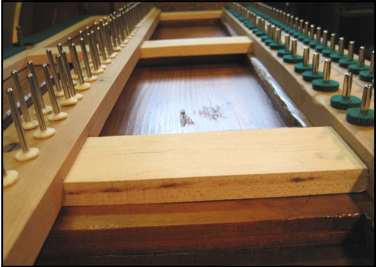
New front and balance rail keypins, ready for the installation of a rebushed set of keys..
