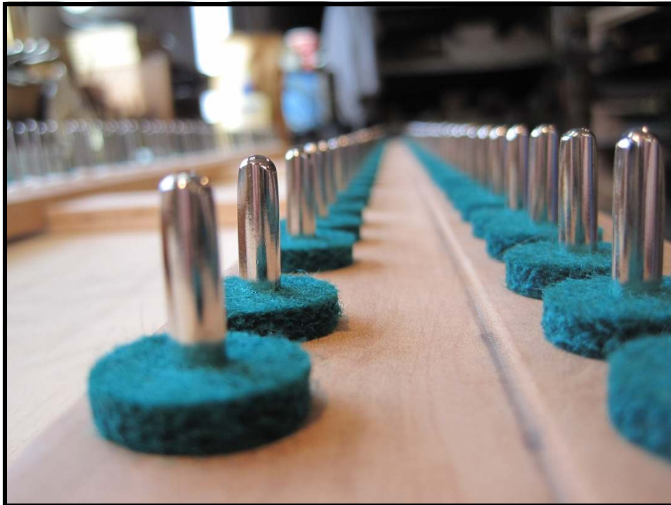
A new set of keypins help give keys a new "feel" when the piano is played.
